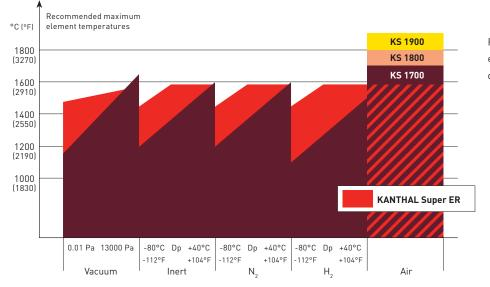
Recommended maximum element temperatures in different atmospheres.
