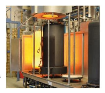
Kanthal alloys offer high creep strengths at temperatures of 1,100–1,300°C (2,012–2,372°F) where conventional metallic materials cannot operate. The performance, energy efficiency and productivity of many high-temperature processes within heat treatment, chemical processing and power generation can be improved by introducing the advanced material technology contained in Kanthal® APMT and Kanthal® APM.
